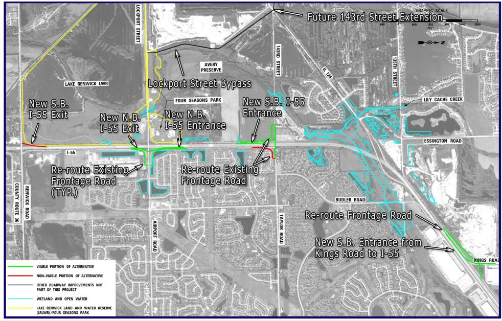
INITIAL ALTERNATIVE 9 - Slip Ramps at Kings Road to SB I-55, at 143rd Street to SB I-55 & at Airport Road to NB I-55. Provide 143rd Street Overpass at I-55. Assume NB I-55 Exit at Airport Road.
