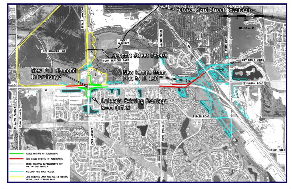
INITIAL ALTERNATIVE 8 - Diamond Interchange at Airport Road & Full Access at IL 126 Interchange with 143rd Street Connector.
