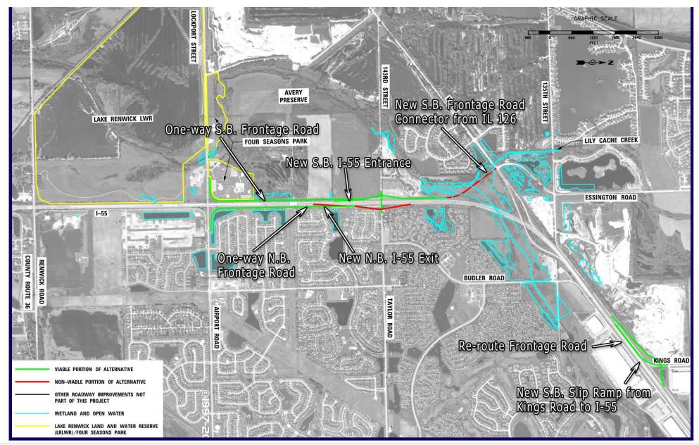
INITIAL ALTERNATIVE 13 - Spread Diamond Interchange at 143rd Street and IL 126. Includes Slip Ramp from Kings Road to SB I-55.
