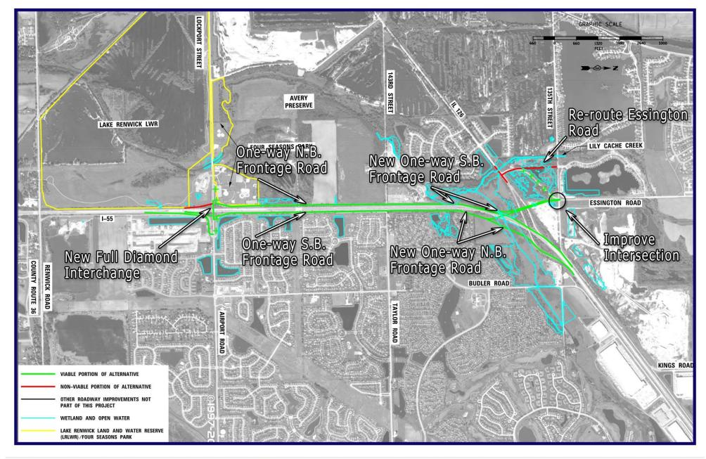
INITIAL ALTERNATIVE 26 - Spread Diamond Interchange at Airport Road & IL 126 with Frontage Road Connection.
