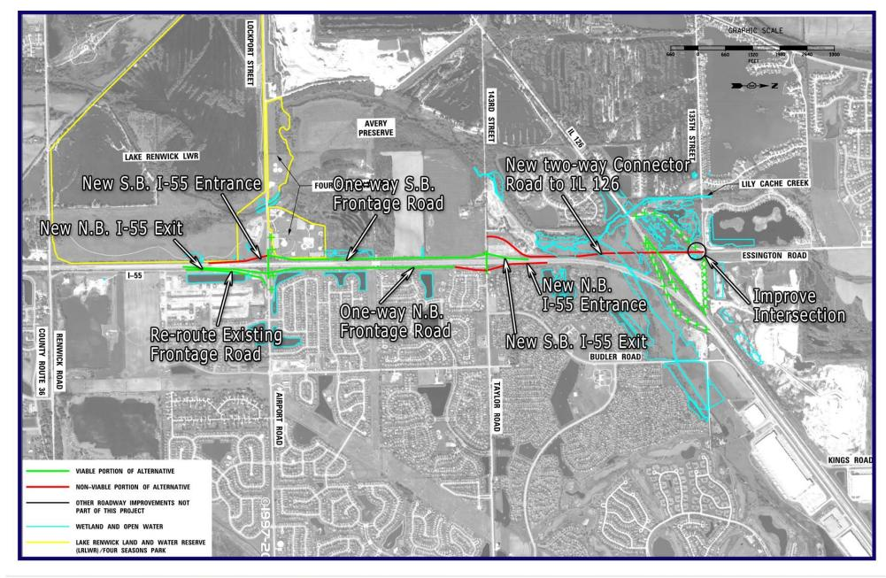
INITIAL ALTERNATIVE 24 - Spread Diamond Interchange at Airport Road & 143rd Street with Essington Road IL 126 Connectors.
