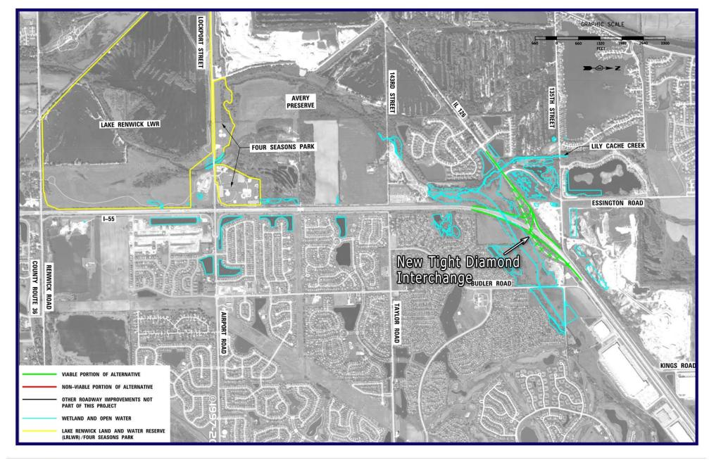
INITIAL ALTERNATIVE 28 - Tight Diamond Interchange at IL 126 with Directional Southbound Ramps.
