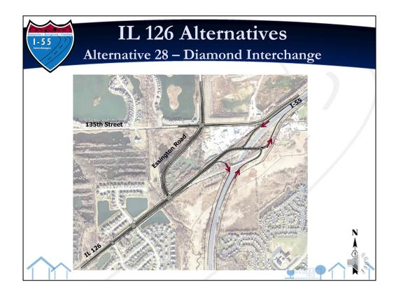
Alternative 28 proposes a Diamond Interchange at IL 126. This alternative will realign ramps to and from the north on I-55 and provide new ramp access to and from the south on I-55. Preliminary screening has found that this alternative will have impacts on wetland areas. Residential and business properties will not be displaced and this alternative will serve future traffic demand with an acceptable level of service.
