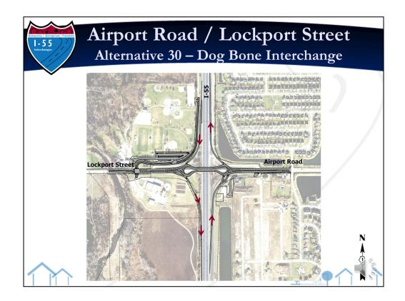
The second alternative located at Airport Road/Lockport Street is Alternative 30, the Dog Bone Interchange. It will provide access to and from I-55 in the northbound and southbound directions.
