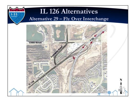
Alternative 29 proposes a flyover interchange at IL 126. This alternative will realign ramps to and from the north on I-55 and provide new ramp access to and from the south on I-55. Preliminary screening has found that this alternative will have impacts on wetland areas. Residential and business properties will not be displaced and this alternative will serve future traffic demand with an acceptable level of service.
