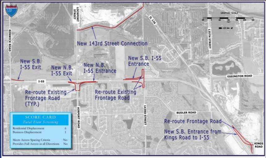
ALTERNATIVE 9 - Slip Ramps at Kings Road to SB I-55, at 143rd Street to SB I-55 & at Airport Road to NB I-55. Provide 143rd Street Overpass at I-55. Assume NB I-55 Exit at Airport Road.
